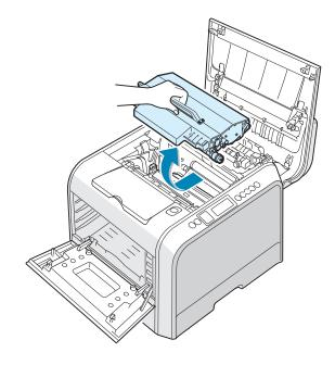
7 Lift the handle of the imaging unit and use it to pull the imaging unit out of the printer. Set it on a clean flat surface.
